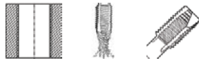
through holes up to 4 x D Chip removal (like picture) Form B with spiral point
