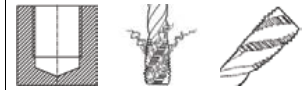
blind holes up to 2 x D Chip removal (like picture) Form C 15° spiral flute
