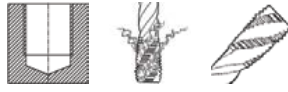
blind holes up to 3 x D Chip removal (like picture) Form C 35° spiral flute
