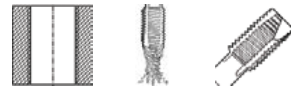
through holes up to 2.5 x D Chip removal (like picture) Form B with spiral point
