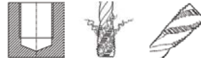
blind holes up to 2.5 x D Chip removal (like picture) Form C 40° spiral flute
