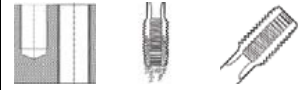
through holes & blind holes up to 2 x D Chip removal (like picture) Form C straight flutes
