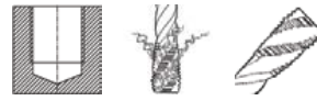
blind holes up to 3 x D Chip removal (like picture) Form C 35° left spir. flute
