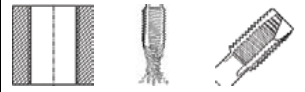
through holes up to 3 x D Chip removal (like picture) Form B with spiral point
