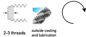
2-3 threads outside cooling and lubrication
