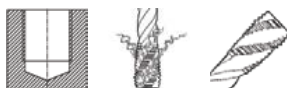
blind holes up to 3 x D Chip removal (like picture) Form C 35° spiral flute
