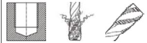
blind holes up to 3 x D Chip removal (like picture) Form C 35° left spir. flute
