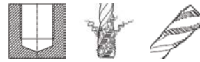
blind holes up to 2.5 x D Chip removal (like picture) Form C 35° spiral flute
